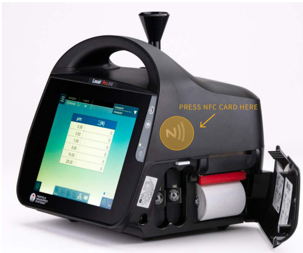
Figure 6-5. Internal NFC card reader location
