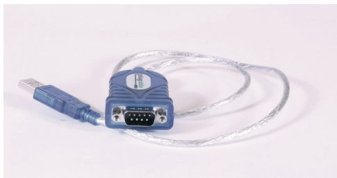
USB to RS-232 Converter PN 1000023262
