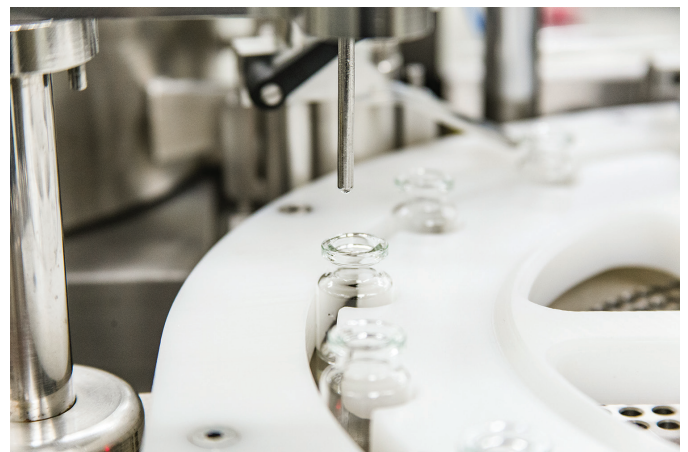
FIGURE L-1 CRITICAL POINT OF A FILLING LINE
