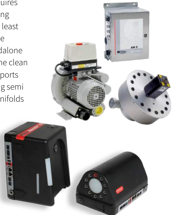
FIGURE 2 AIR MANIFOLD 16 PORT SYSTEM (TOP, GREY INSTRUMENTS) AND NANOAIR & PARTICLESEEKER SYSTEM (BOTTOM, BLACK INSTRUMENTS)
