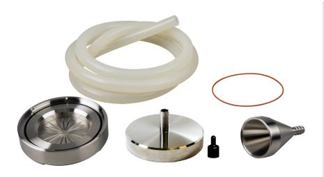
When remote and flexible monitoring with no fixed sampling point is needed, the Remote Sampling Isokinetic Sampling Probe (ISP) Kit allows for samples to be taken while maintaining the integrity of the measurement. The ISP Kit uses a length of sample tubing to connect the sample point to the impaction plate, and is ideal for minienvironment sampling applications such as RABS, Laminar Flow Cabinets and Blow-Fill-Seal/Form-Fill-Seal settings.
