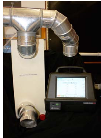
Figure 2 Lasair III 5100 reference unit beneath a HEPA air supply
