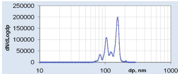
Figure 5. A typical PSD obtained with NaCl particles fractionated using the Naneum DMA model PMC500 configured for mobility equal to 150 nm for a singly-charged particle. The sample aerosol was charged with a K_r source and recorded with the NPS500 Nanoparticle Spectrometer neutralizer.
