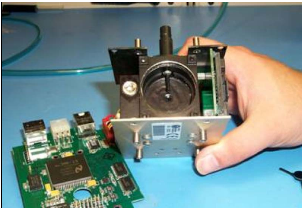
Figure 2. Teflon-coated Airnet-510 XR optics chamber and internal components.
