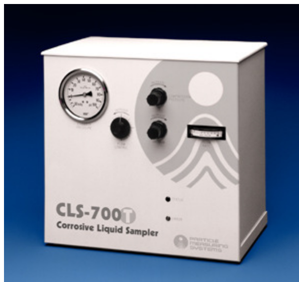
Figure 6: The CLS-700T is an example of a bubble compression system.
