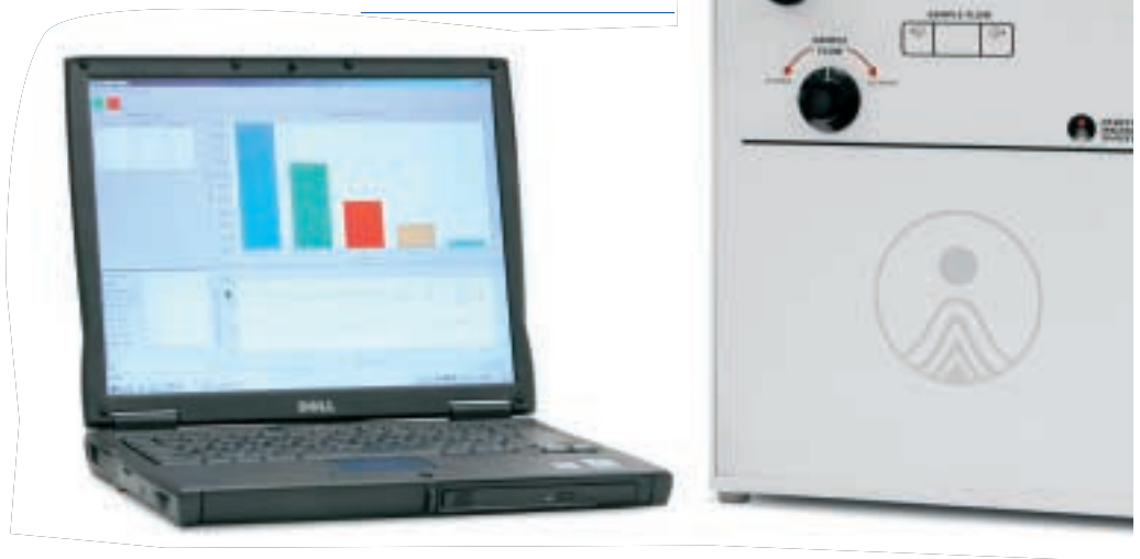
Fig. 1: Example of a liquid compression sampler and PC used for control and data collection
