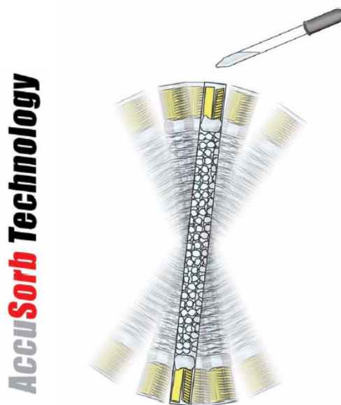
Figure 16. AccuSorb Technology Ultrasonic Extraction with 3 ml of solvent
